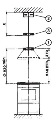
Note: If the hood is to be installed onto a hollow construction or plaster or partition board wall then special fixing screws will be required (not supplied).
